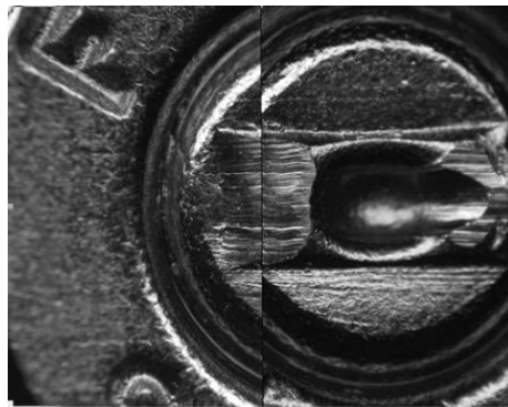
Image 2. Side-by-side microscopic comparison of two cartridge casings; the thin vertical black line divides the two casings. The casings are oriented to compare toolmarks (breech face marks and firing pin impression). 59 It is easy to see superficial similarities, which are not necessarily indicative of a shared source.
