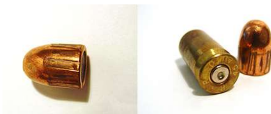
Image 1. Discharged bullet (left) and discharged cartridge case and bullet (right). Striations on the bullet’s surface and the firing pin impression on the casing are visible to the naked eye. 56
